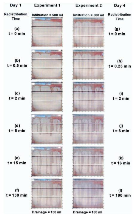
Fig. 2. Photographs of the wetting front taken at different times (a-f) during redistribution in dry sand and (g-l) during second cycle of redistribution with fingers in the sand. The redistribution time is indexed from t = 0, defined as the moment when ponded water first disappeared from the sand surface.
